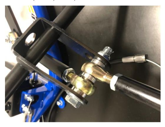
Now is the time to go over all of the front end adjustments to make sure they are correct and all the hardware it tight. First, align the caster block with the welded caster plates to the
